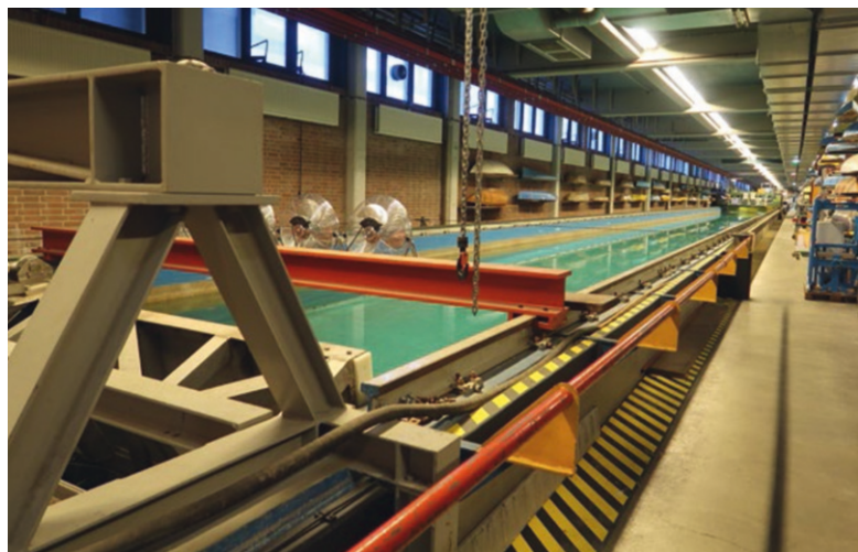
↑The long towing tank of the TU Delft today, with tested models on the wall. Besides the long and the small towing tanks for research, a much smaller tank is in use today, mainly for the training of students. It has been named Bruno, after the towing tank pioneer Tideman (see § 2.3.1).
