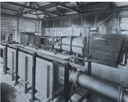
↑The towing tank/water tunnel/wave flume in Burgers' laboratory in Delft around 1930. (courtesy of Burgers Archives / Delft University of Technology)
