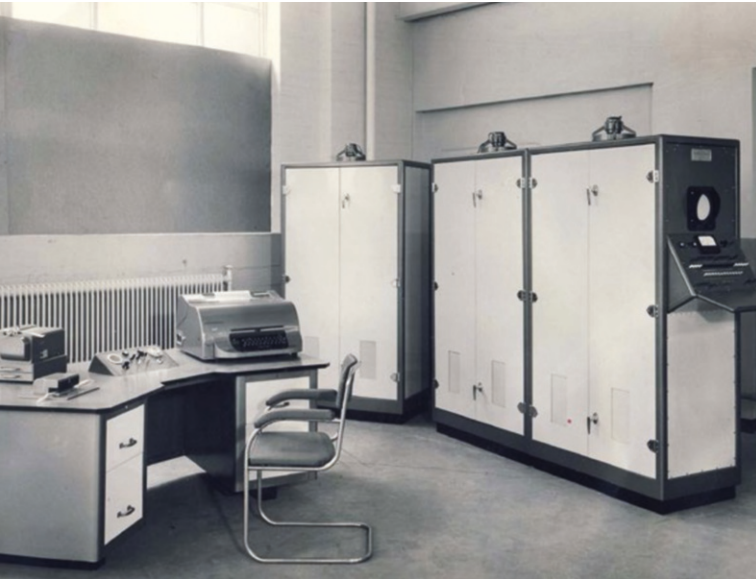
The first computer of the NLL, the ZEBRA, was used from 1958 for data reduction of the High Speed Tunnel. (courtesy of Stichting Behoud Erfgoed NLR)
