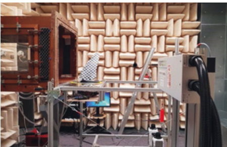
↑The open jet test section of the wind tunnel in Twente is located inside of a large anechoic chamber which has dimensions 6 \times 6 \times 4 m. Here research is done on the vortex generated by the flapping wing of a robotic bird. (courtesy of Kees Venner / University of Twente)
