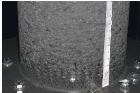
↑→ The bubble column in Delft as it is today. It was the first in its kind with so many needles and such large diameter. Besides, the bubble flow remained uniform for a long time; only at a volume fraction of 55 percent the water started to circulate. (courtesy of TU Delft / Rob Mudde)
