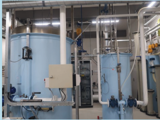
↑ In one of VSL's so-called bell provers the Dutch cubic meter is born. This is the primary gas flow measurement standard in the Netherlands. Calibrations of flow meters using the left bell prover have a measurement uncertainty of below 0.1%. (courtesy of VSL / photo by Fons Alkemade)
