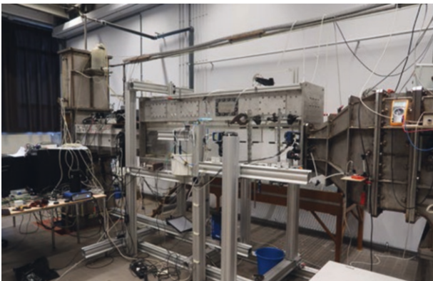
↑The cavitation/water tunnel of the TU Delft as it is today. Here research is done on drag reduction by means of air lubrication along a flat plate. Measurements are performed with PIV.
