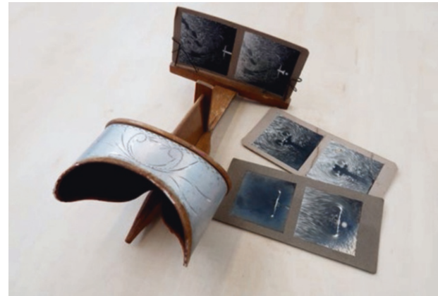
↑During Burgers' experiments on flows behind objects in the small towing tank, also stereo photos were made. These were taken by a camera moving along with the objects. (courtesy of Burgers Archives / TU Delft)
