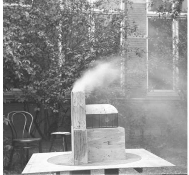
↑ Flow visualization in the 1930s. Around 1936 a temporary 'shed' was built close to Burgers' Laboratory for experiments on the ventilation channels of the Maastunnel (see § 3.4.3). Parts of the model were made transparent and strings were placed inside which would follow the air flows. On the left one sees one of the many Betz precision manometers which were then used in the laboratory. Outside the building a model of the complete ventilation building was tested using smoke. (courtesy of Burgers Archives / TU Delft)
