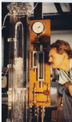
↑→ The bubble column in Delft as it is today. It was the first in its kind with so many needles and such large diameter. Besides, the bubble flow remained uniform for a long time; only at a volume fraction of 55 percent the water started to circulate. (courtesy of TU Delft / Rob Mudde)
