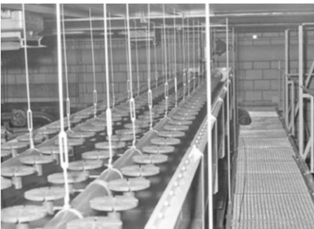
↑The sloping flume in Wageningen around 1971, with the 'rain simulators' above it. (courtesy of Wageningen University & Research)
