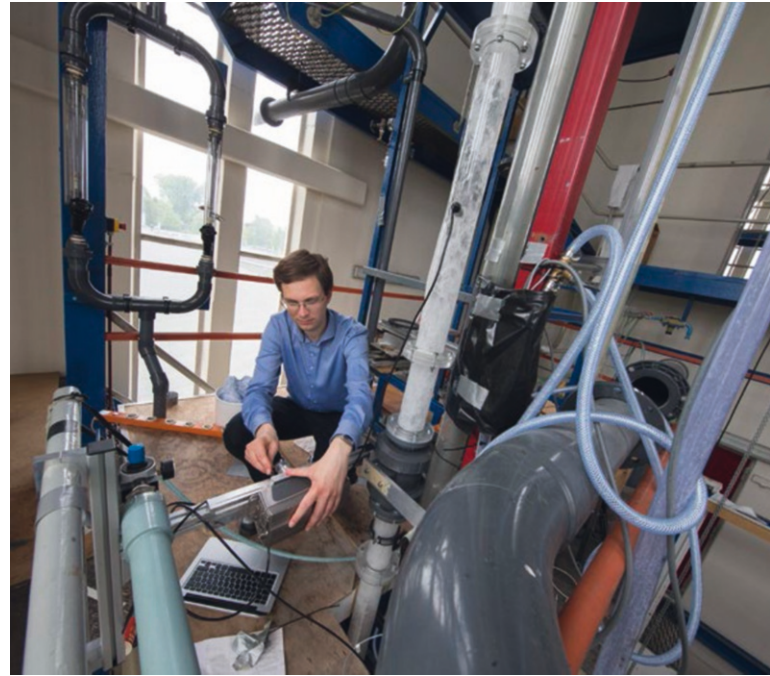
↑ ‘Severe slugging’ research as presented in a PhD thesis published in 2012 (supervised by professor Rob Mudde of the Kramers Laboratory) including experiments in this large facility (the Severe Slugging Loop) at the Shell Technology Centre in Amsterdam in which slug flow in a flowline-riser system could be investigated (from: Malekzadeh (2012); courtesy of TU Delft).
