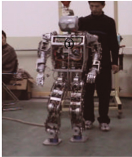
Fig. 5. BHR-1 walked in 2002 at a speed of 2 km per hour
