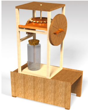
Fig. 9. Figure 30 assembly, water clock
