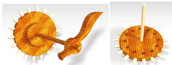
Fig. 7. (a) Main shaft and water clock hand. (b) Ball wheel with holes for balls
