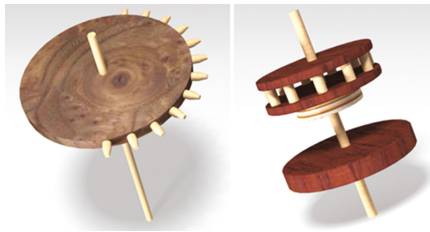
Fig. 5. Main and secondary shaft of the mechanical well
