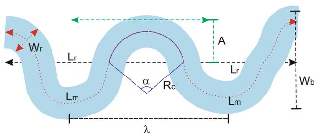
**Fig. 29.6** Geometric elements of a meandering channel pattern that are generally used in mathematical calculations and formulations of the meandering ratio, curvature or other approaches (modified from Güneralp and Marston 2012).  $L_r$ —Straight length,  $L_m$ —Sinuous channel length,  $\alpha$ —Arc angle,  $R_c$ —Radius of curvature,  $W_r$ —Width of river,  $\lambda$ —Linear wavelength,  $A$ —Meander amplitude,  $W_b$ —Belt width ( $2A$ )
