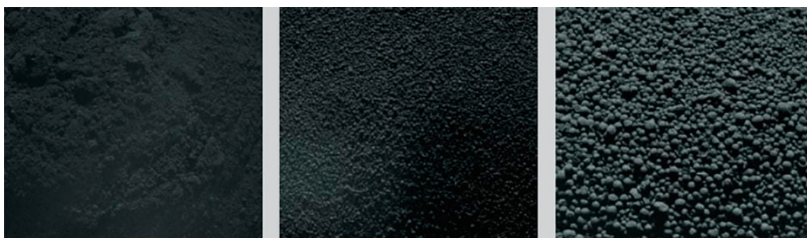
Fig. 5.10 From left to right: powder carbon black, dry-pelletized carbon black, wet-pelletized carbon black. (Reproduced with permission of Orion Engineered Carbons )
