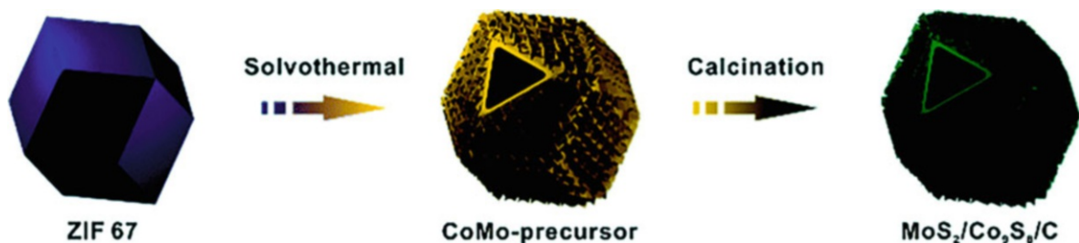
Fig. 4.113 Illustration of the formation of the MoS 2 /Co 9 S 8 /C nanobox by a solvothermal method and a subsequent calcination process. (Reproduced with permission of the Royal Society of Chemistry )
