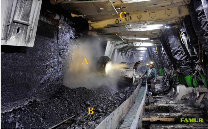
Fig. 1. Longwall machinery ( https://famur.com/upload/2016/09/FAMUR_01-1.jpg )
