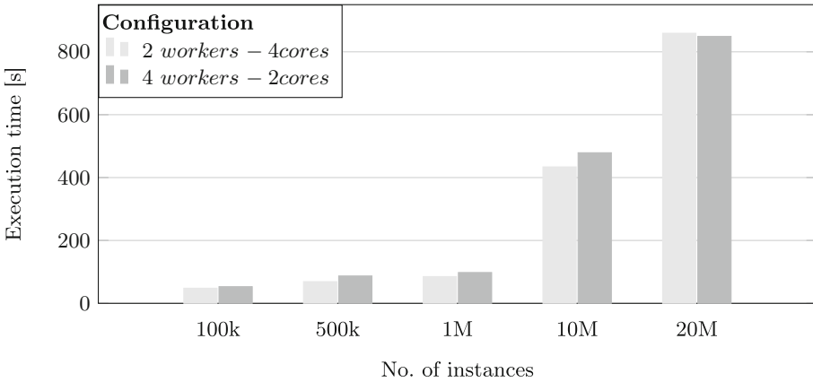
Fig. 1. Comparison between execution time for a cluster made of PCs with 2 core CPUs and 4 Workers and a cluster with 2 Workers and PCs with 4 core CPUs
