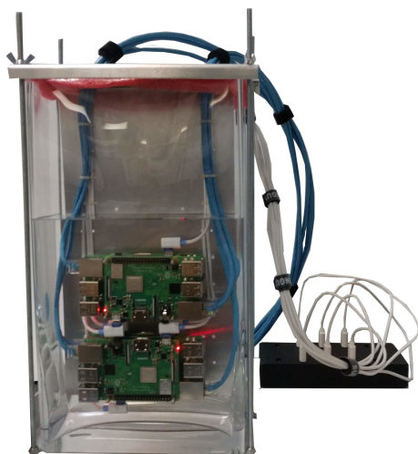
Fig. 2. HFE-based immersion cooled prototype.
