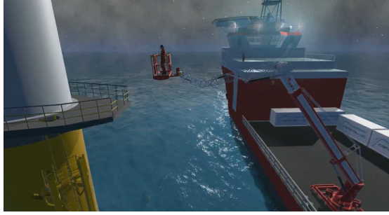
Fig. 3. 3D real-time simulation of a motion compensated crane. Taken from [14].
