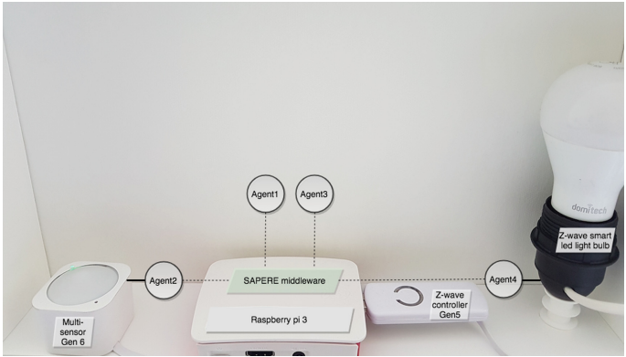
Fig. 7. IoT node implementing our scenario
