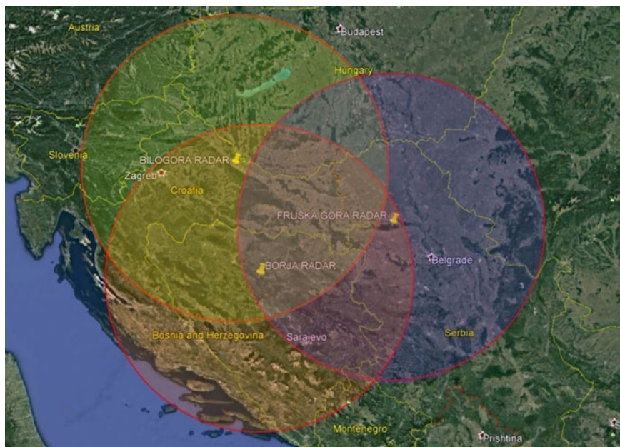
Fig. 2 Radar coverage by meteorological radars in Borja (B&H)—yellow, Bilogora (Croatia)—green and Fruška Gora (Serbia)—blue, within 200 km observation reach
