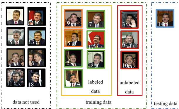
Fig. 2. Illustration of how the data is divided. In this experiment, firstly, the data is randomly divided into 3 parts during the whole training process. Secondly, for training data, we randomly select 2 of them as the initial labeled data (i.e., orange frame) and the rest as unlabeled data. Then, we gradually add the labeled data (i.e., green frame) from the rest of the unlabeled data (i.e., red frame) via AL algorithm to boost our model. After all, we use testing data to test our model. (Color figure online)
