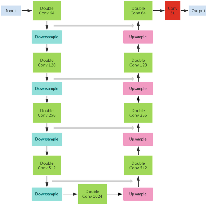
Fig. 1. Diagram of the proposed method. “Conv m ” represents convolutional layers with an output of m feature maps. We use 3 \times 3 convolution in green blocks and 1 \times 1 convolution in the red block. Gray arrows represent feature concatenation (Color figure online).
