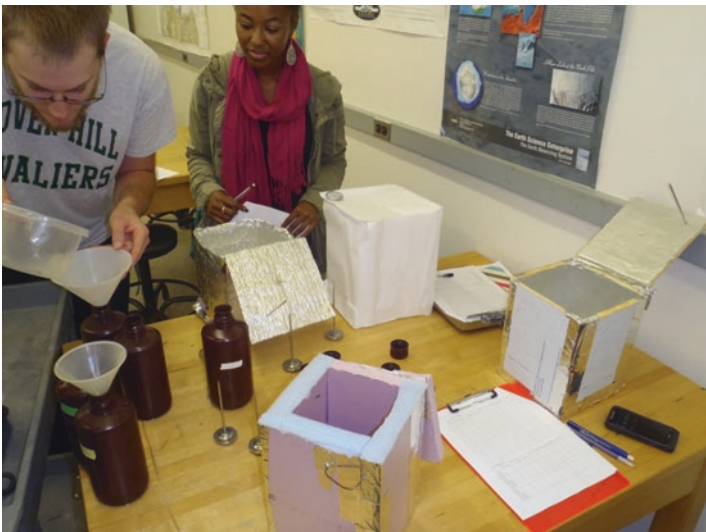
Fig. 3 Students use simple and inexpensive materials to test the effectiveness of different types of commercially available insulation and calculate rates of heat transfer
