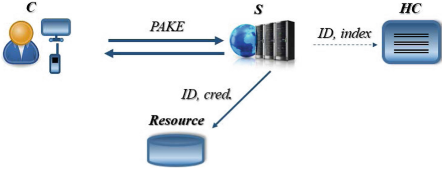
Fig. 2. HoneyPAKE system. The client wants to use the Resource. After running the HoneyPAKE protocol with the login server S , the client can access the resource. The credential shared between the Resource and C can be the output of the HoneyPAKE.
