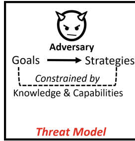
Fig. 3. Template to define a complete threat model. Adversary goals are used to define attack strategies while being constrained by the knowledge and capabilities of the adversary.
