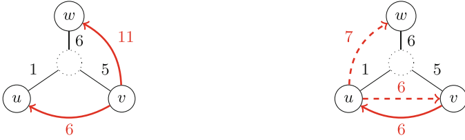
(a) An example configuration: v has u and w in its local memory. Note that u and w are neighbors of each other in the MST.
