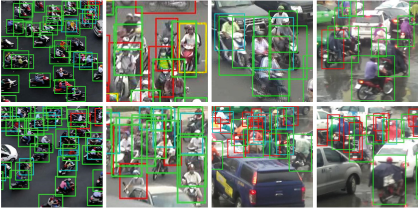
Fig. 6. A few detection results on three datasets. For visibility, only results on motorbikes are drawn. These images are also zoomed in and cropped. Green box: true positive, blue box: false positive, red box: false negative. (Color figure online)
