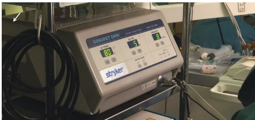
Fig. 4.6 Ultrasonic aspirator. Console showing values of power, suction, and irrigation (Sonopet®, Stryker, Kalamazoo, MI, USA)
