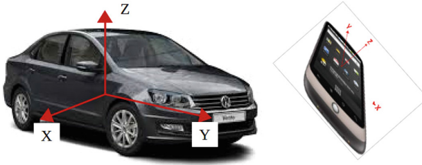
Fig. 5. The coordinate system of the car and of the phone do not coincide.
