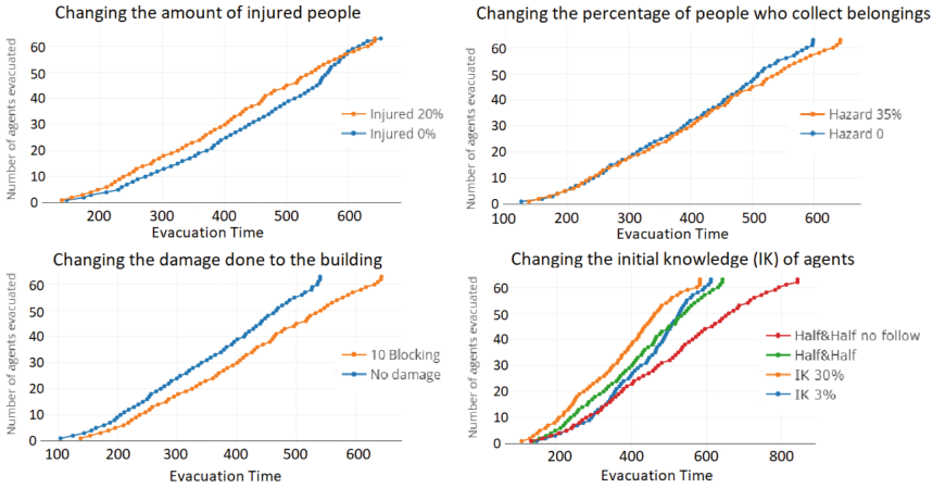
Fig. 6. The average number of agents evacuated after the quake for the university environment. Evacuation times are measured in seconds.
