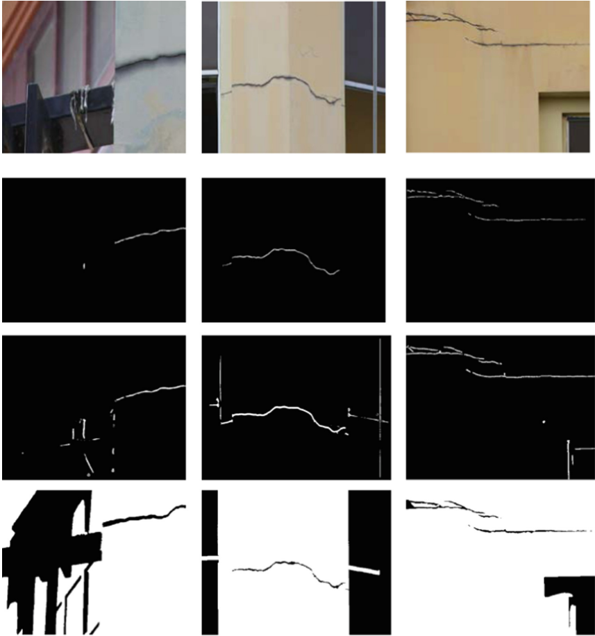
Fig. 8. Comparison between proposed method, Fujita's method [9] and Hutchinson's method [20]. From first to fourth row: input image, binary image result from the proposed method, result of Fujita's method, result of Hutchinson's method.
