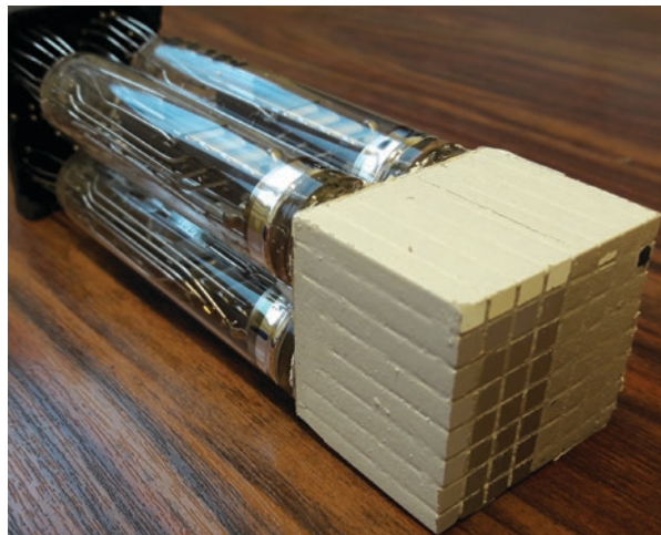
Fig. 2.1 ECAT EXACT HR+ (Siemens) detector block composed of 64 crystals and read by 4 PMTs
