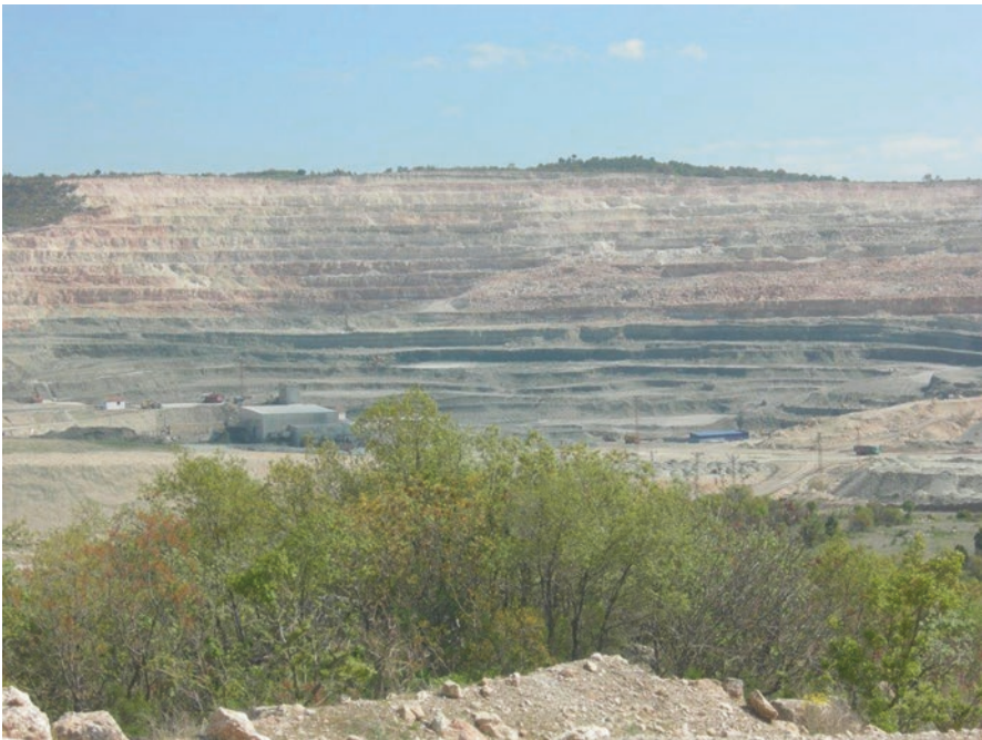
Fig. 11.18 Section of borate zone interbedded with clay and tuff, and limestone overburden, in the opencast mine of the Espey deposit, Emet, Turkey
