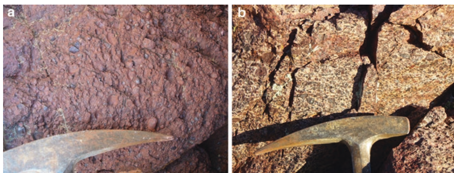
Fig. 15.27 The Öşün bauxite ore has pisolitic-oolitic textures with different colours, such as (a) reddish-brown and (b) white matrix with dark pisolites
