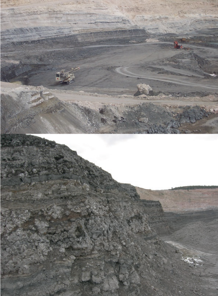
Fig. 11.33 Hisarcık open cast mine showing borate zone and limestone overburden, Emet area, Turkey
