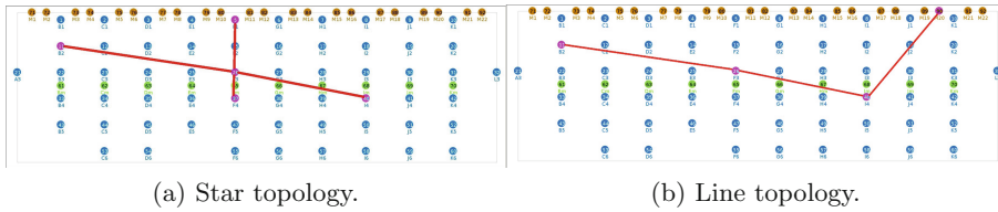
Fig. 2. Logical topologies from Fig. 1 mapped onto physical nodes in w-iLab.t .
