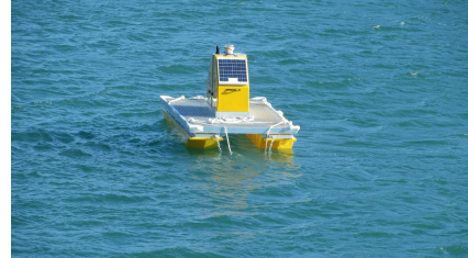
Fig. 2. Avoid hard-accessible places, if possible. To achieve this platform, the technicians needed about 45-min boat drive. They installed the platform (incl. motes and a GSM modem) but had to come back here after a few days only to update software.
