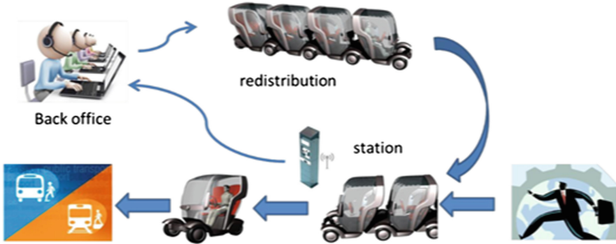
Fig. 1. The architecture of an ESPRIT-based car-sharing system [13].
