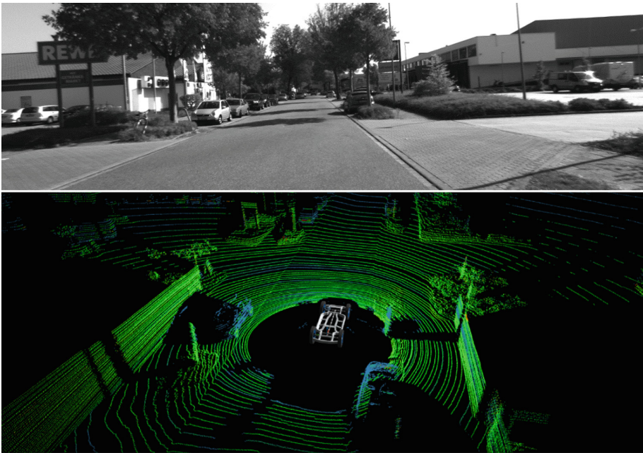
Fig. 10. Camera image (top) and raw point cloud (bottom) of the first test-scene.
