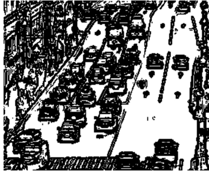
Fig. 8. Video frame with application of edge detection algorithm and binarization
