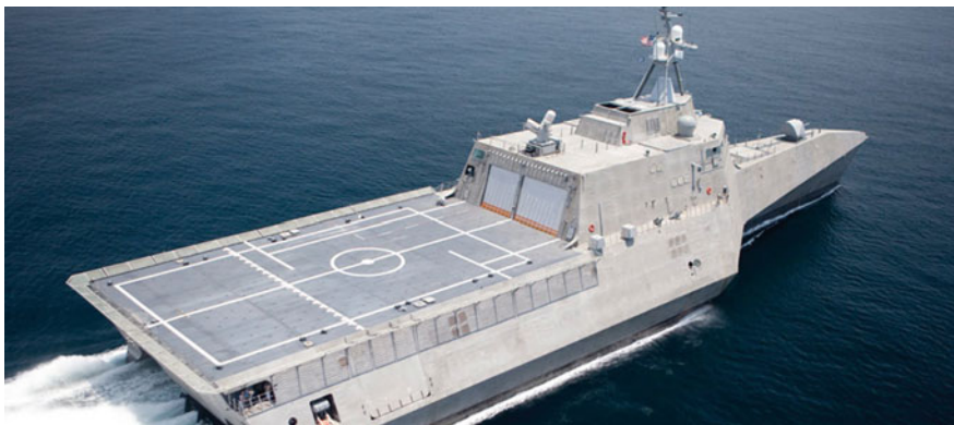
Fig. 10.6 Littoral Combat Ship is an example of bus modularity, where different mission modules, packaged as containers, can be plugged into a standard interface to provide a wide array of different mission capabilities (AOC 2018)
