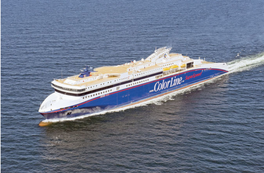
Fig. 4.1 RoPAX vessel «MS Colour Superspeed 2», delivered 2008, a fast ferry with passenger spaces for day travellers. Capacity: 1928 passengers and 2034 lane metres ( http://www.faktaomfartyg.se/superspeed_2_2008.htm )
