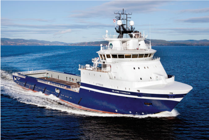
Fig. 4.3 Typical offshore supply vessel (OSV) type RR UT 776 «MS Island Condor», delivered 2014, 4700 dwt ( https://www.islandoffshore.com/fleet/fleet-overview/psv )
