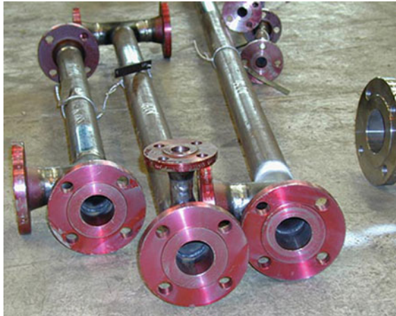
Fig. 10.7 Ship piping system, illustrating sectional modularity (Erikstad 2009)
