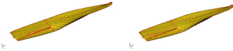
(C) Panel meshes for seakeeping analysis (input to NEWDRIFT+)
