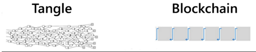
Fig. 1. Visual display of the different between a DAG (the Tangle) and a blockchain - image reprinted from [14]
