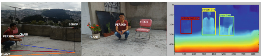
Fig. 7. Test with obstacles at a short distance from the micro-UAV. Although the person is squatting, the model recognizes him.
