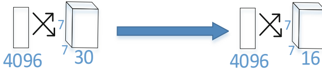
Fig. 6. Original YOLO Net. It divides the image into an 7 \times 7 grid and for each grid cell predicts 2 bounding boxes, confidence for those boxes, and 3 class probabilities and another 3 angle information. These predictions are encoded as an 7 \times 7 \times (2 \times 5 + 3 + 3) = 7 \times 7 \times 16 tensor.
