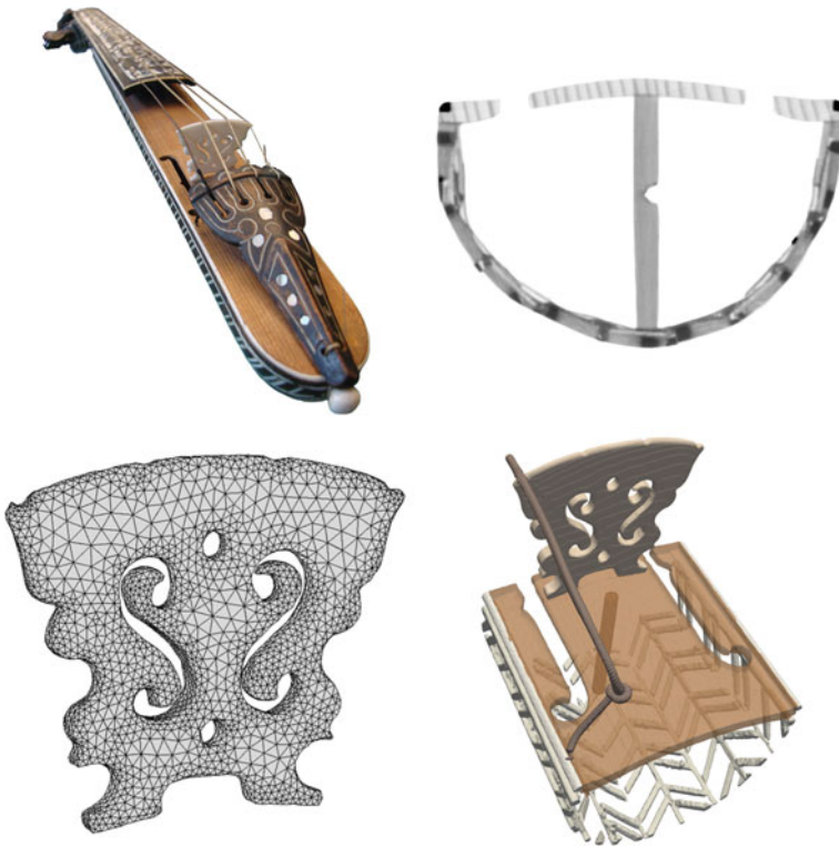
Fig. 3 Exemplary results of the proposed workflow (clockwise): photo of a 17th century kit violin, cross-sectional CT image (inverted grey values), rendering of sub-structures after segmentation, finite element model generated from the bridge sub-volume. The original instrument is on display at Germanisches Nationalmuseum Nürnberg, Germany. The CT data has been acquired by the MUSICES project [24]
