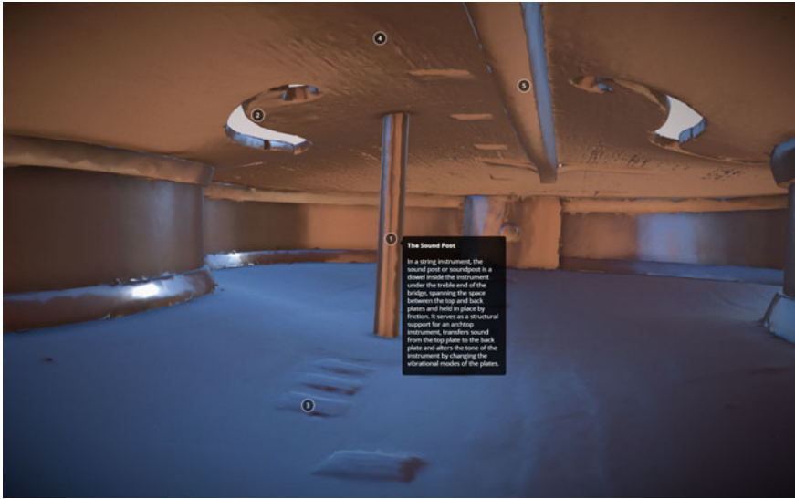
Fig. 5 VR view into the rendered inner part of a viola. The observer can “walk” through the instrument, individual parts are annotated to explain their functionality. The model is based on an X-ray CT scan, the rendering is generated with the VR viewer from Sketchfab. Exemplary annotation text retrieved May 4, 2018, from https://en.wikipedia.org/wiki/sound_post
