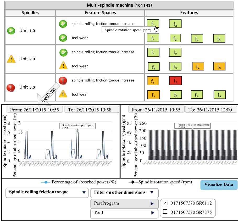
Fig. 4. Visualisation of relevant data on operator’s cockpit in the anomaly detection application scenario (GetData method).
