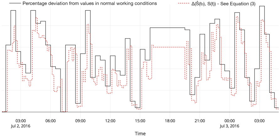
Fig. 6. Correlation between the value of the percentage deviation from the values of rpm and absorbed power features in normal working conditions (black line) and the value of \Delta(\hat{S}(t_0), S(t)) computed according to Eq. (3) (dashed red line) (Color figure online).
