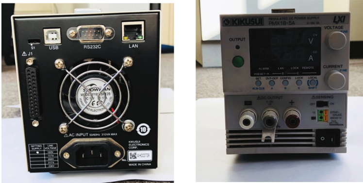
Fig. 4. The voltage meter in the prototype system. As shown in the left figure, the given voltage can be controlled through the RS232C, USB, or LAN.
