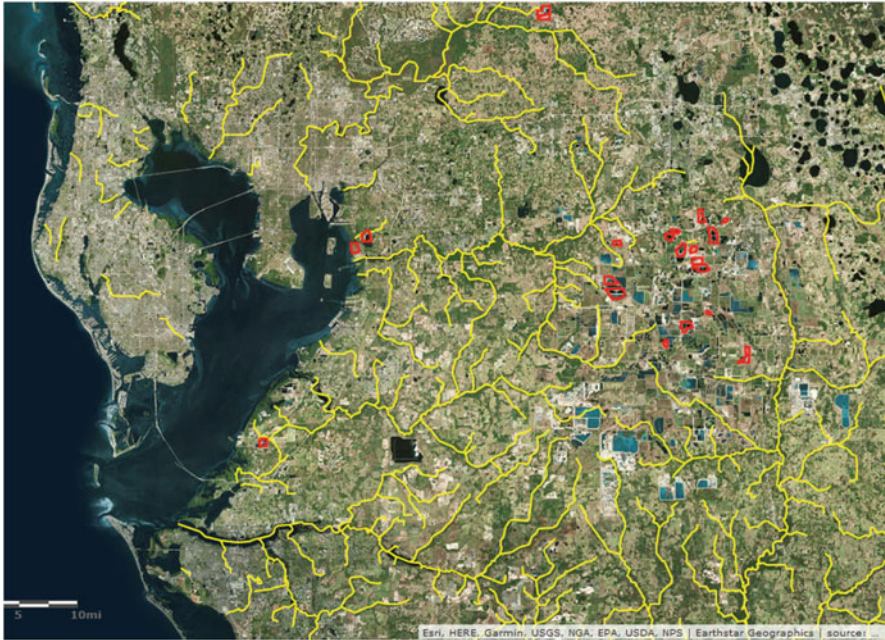
Fig. 5.19 Phosphate mining areas (blue), waterways (yellow) and gypsum stacks (red). (FDEP 2011)
