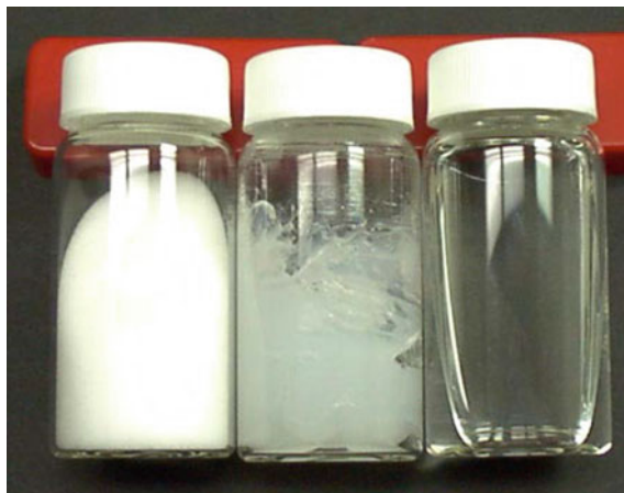
Fig. 10 Picture of POSS materials, fully condensed octaisobutyl T_8R_8 (left), polyethylene glycol (PEG, chain length C_n = 10 ) T_8 POSS (center), fully condensed octaisooctyl T_8R_8 (right)
