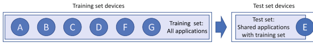
Fig. 1. Leave-one-out training- and test-set splitting: inspired by k-fold cross-validation, we leave the binary executables from one device as test-set out, while applications from all other devices constitute the training set. The test-set contains only applications where a record is present in the training set (shared applications), while the training set contains all records irrespective of the application’s presence in the test-set.
