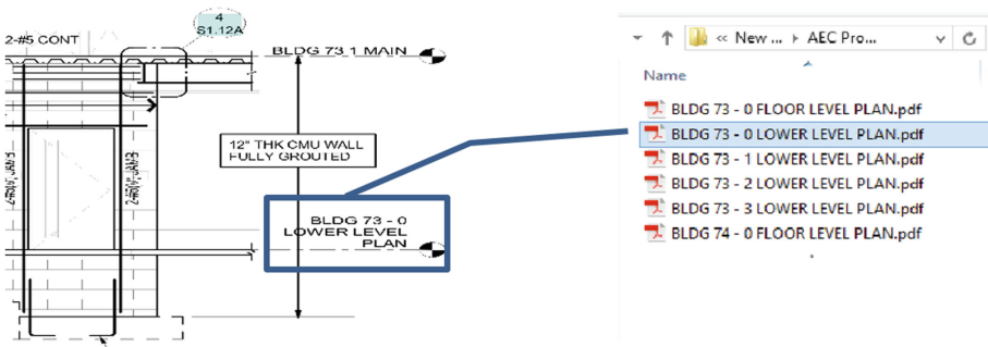
Fig. 8. Hyperlink navigation representation; When clicked on the Elevation Datum shape of a document, it will automatically navigate to the associated document i.e. BLDG 73 – 0 LOWER LEVEL PLAN .
