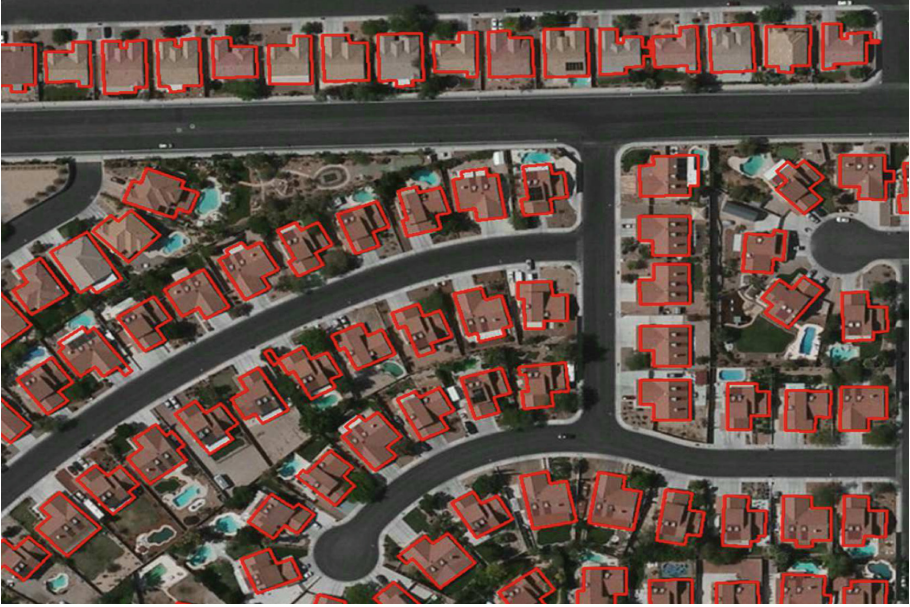
Fig. 10. The red polylines are the resultant orthogonal shapes. The result is overlapped with imagery to evaluate quality of the method. (Color figure online)
