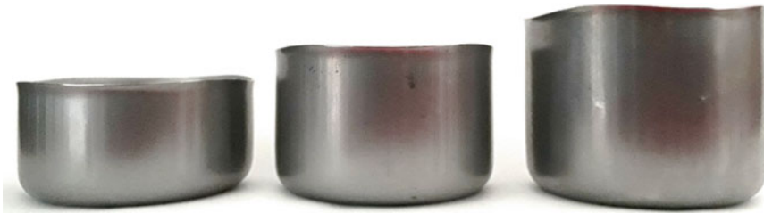
Fig. 7 Cylindrical cups obtained for DP780 material using a blank diameter of 105, 115 and 125 mm (left to right, respectively)
