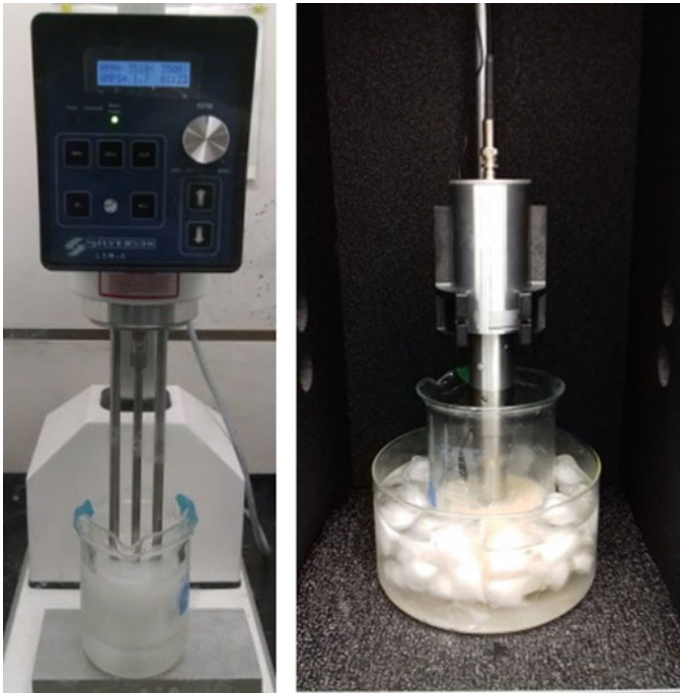
Fig. 2 Mixing (left) and sonicating operations (right)
