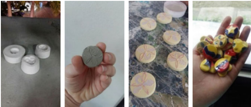
Fig. 10 Full manufacturing process: plaster molds, Barbotina's pieces, pigmentation process, cooking (left to right)
