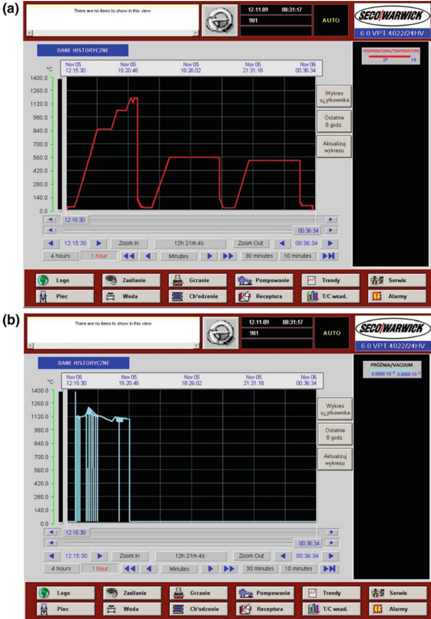
Fig. 2 Run of heat treatment of cutting edges in SECO/WARWICK 6.0VPT-4022/241QHV vacuum furnace [13]. a The red line—temperature, b the green line—pressure
