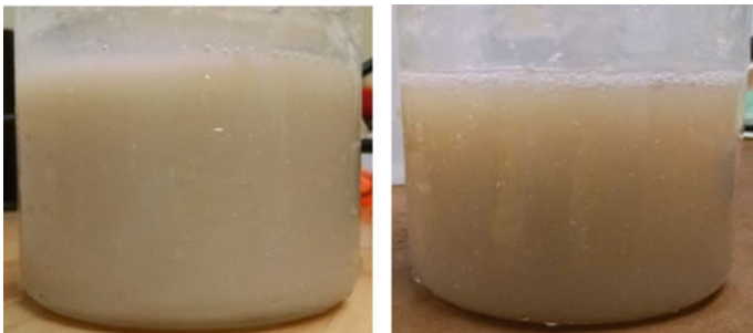
Fig. 3 E/WA/C mixture before (left) and after (right) the sonicating process
