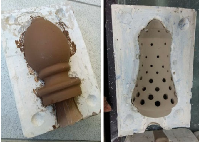
Fig. 8 Gray and Black Barbotina's pieces in blaster molds
