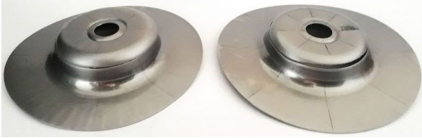
Fig. 9 Fracture experimental cases when the critical blank diameter was exceeded (DP780 using the blank diameters of 135 mm and 130 mm, left to right, respectively)
