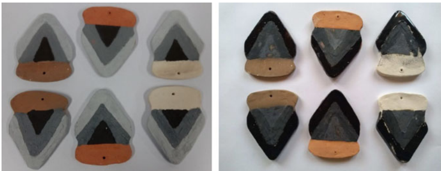
Fig. 7 Comparison between pieces with one and two cooking process
