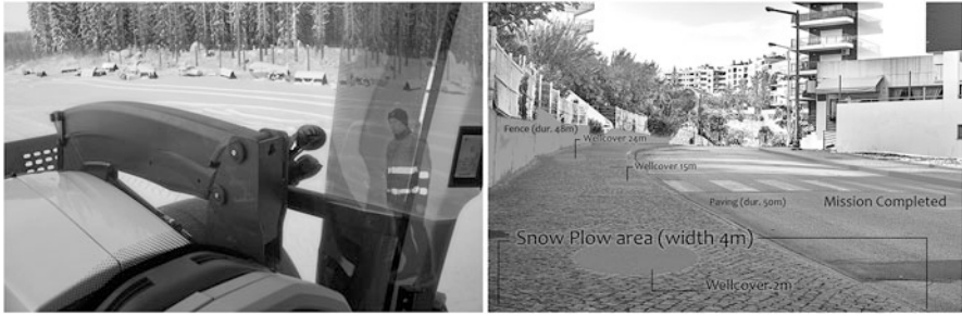
Fig. 2 Left: With transparent tractor pillars, it is easier to observe people in proximity of the machine. Right: Static information about the plowing area is projected to the driver
