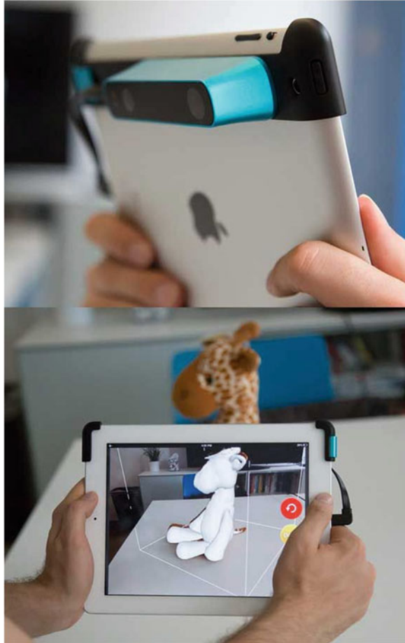
Fig. 4 A Structure IO scanner, manufactured by Occipital, is attached to an Apple iPad device. Loaded with the Structure app, a real world object can be scanned into a digital 3D format as .OBJ, .FBX or .STL files that can then be uploaded to the Sketchfab website to view in VR via a mobile device and a Google Cardboard compatible VR headset
