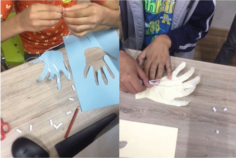
Fig. 7 One of the prototypes developed was a robotic hand, using paper, straws, tape and rope
