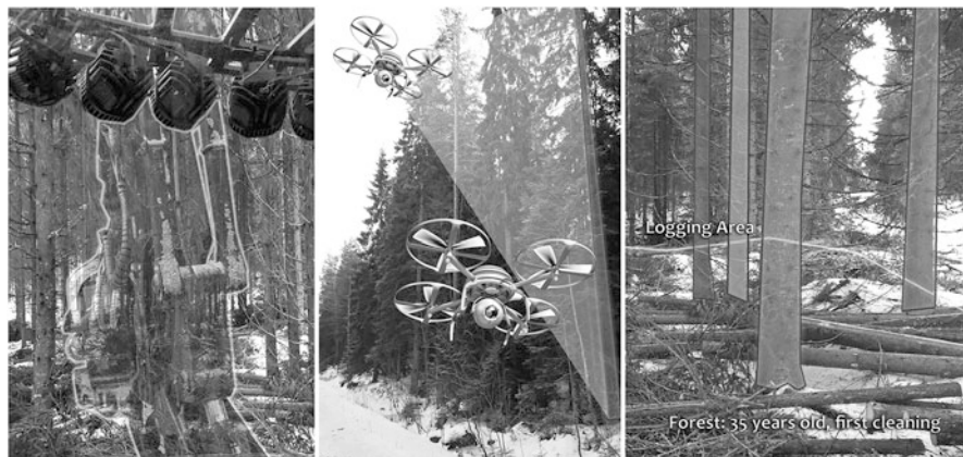
Fig. 3 Left: semi-transparent harvester boom; Center: areal drones inspecting the forest conditions; Right: color-coded guides for indicating the conditions of trees
