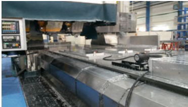
Fig. 8.11 Validation of diagonal error measurement test: a laser tracker installed in GEPRO 502 machine; b example showing the measurement points needed for the complete volumetric characterization (blue) and the diagonal measurement (red)
