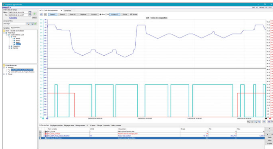
Fig. 8.5 Example of machining step decomposition. In blue, Z-axis position; in red, the tool changes; and in green, axis moving conditions
