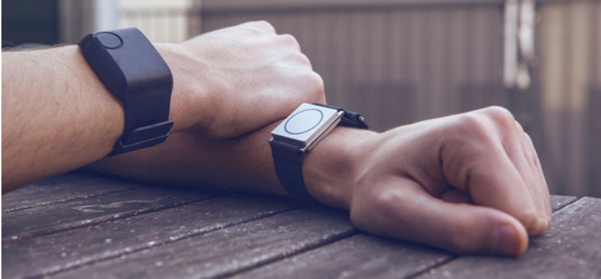
Fig. 6.5 On the left, Empatica E4 wristband research device; on the right Empatica Embrace device with patented technology to continuously record physiological signals from multiple sensors and generate seizure alert
