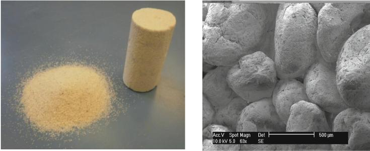
**Fig. 2.** Typical example of bio-treated sand (left) and its SEM image (right)
