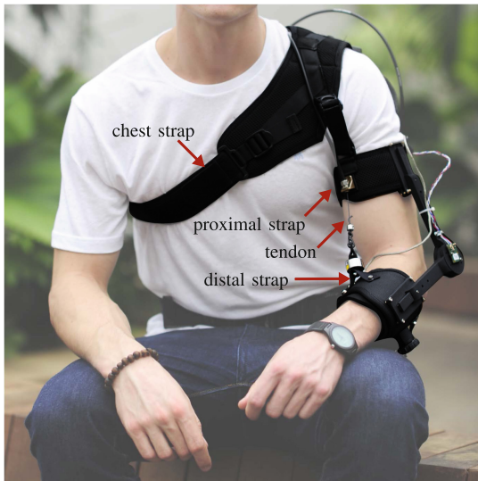
Fig. 1. The soft exosuit for assistance of the elbow joint. Pressure distribution measures were taken at the interface between the distal strap and the skin. Photography by © Stefano Mazzoni.
