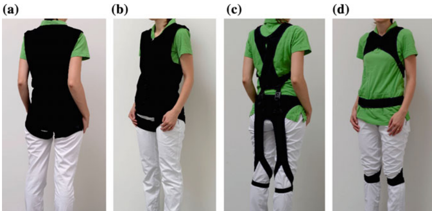
Fig. 1 Suit A (a and b): crossed belts beneath the vest are stretched when bending the torso forward. Suit B (c and d): crossed belts on the back and belts behind the thighs are stretched when bending the torso and knees
