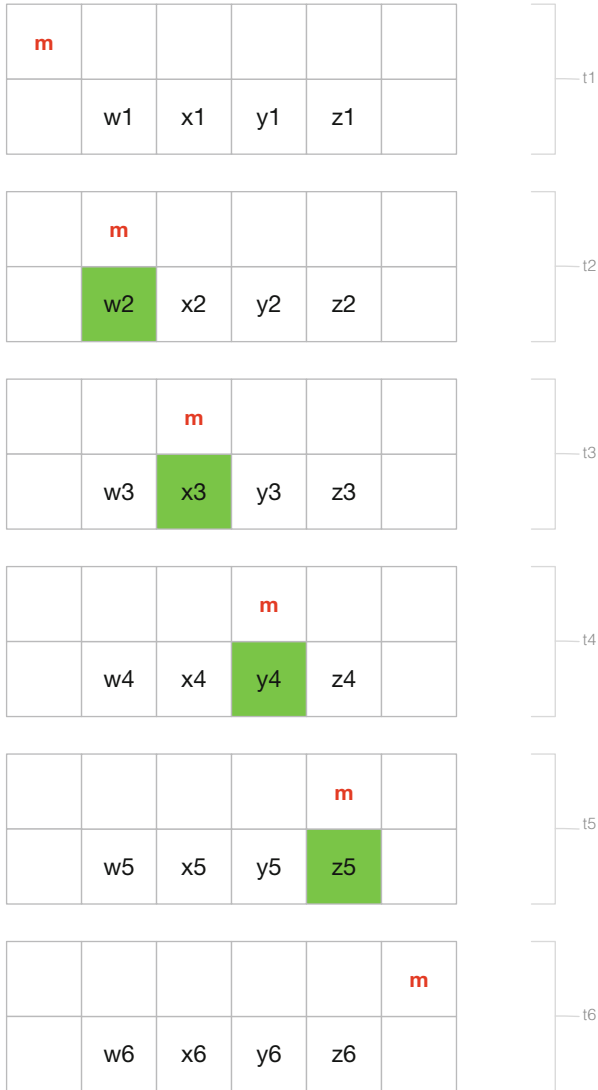
Fig. 13.3 One interpretation of the sensory data. The sensors ( w, x, y, z ) are shown at each time step. E.g. w1 means sensor w at time step 1. The interpretation that the Kantian machine finds is that there is a moving object, m , moving from left to right, in the row above the sensors. The moving object turns on the sensor when the mover is directly above the sensor. Note that the moving object is not directly perceived; it is constructed (or invented) to make sense of the data
