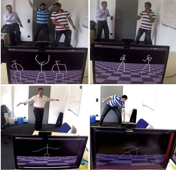
Fig. 6. The real-time 3D pose estimation with Implementation 1 (Top) and Implementation 2 (Bottom). Our algorithm provides a natural motion interface on images from live webcam video.
