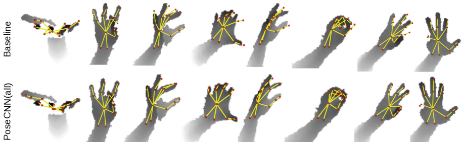
Fig. 3. Qualitative evaluation of our PoseCNN. The top row shows the predicted hand joint positions overlaid on the preprocessed NYU depth images from our baseline implementation (i.e. PoseCNN( J )). The bottom row shows the corresponding images with corrected joint positions from our PoseCNN( all ) implementation.
