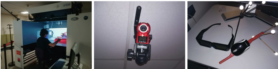
Fig. 1. Aparatus, from the left: Mihriad CAVE, Optitrack camera, tracked glasses and controller
