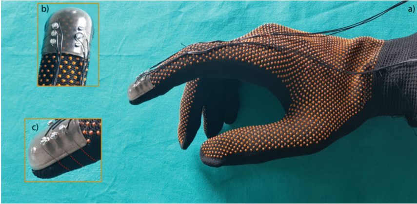
Fig. 2. (a) Early prototype of a tactile glove. (b) Detail of fingernail-shaped support with the electric wires. (c) Detail of the SMA wires stitched on the glove.
