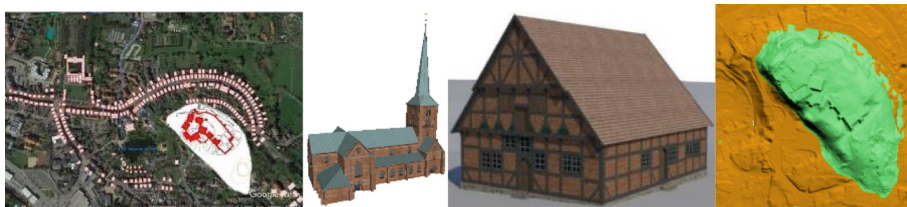
Fig. 3. Positions of historic buildings of Segeberg in Google Earth (left), detailed reconstructed church St. Marien and Old-Segeberg Town House (centre), reconstructed model of the historic lime mountain and its integration in the latest terrain model (right).
