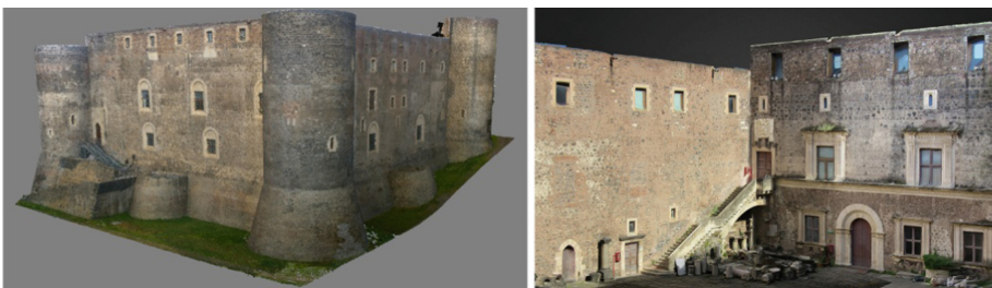
Fig. 1. View of the 3D textured models of the exterior and the courtyard of Castello Ursino.
