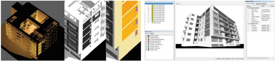
Fig. 6. From left, semantic structure and segmental mesh model, CityGML model (Residential building “Casa Rustici”, Milan)
