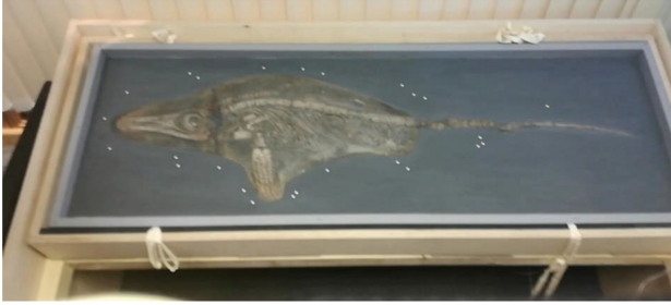
Fig. 3. Image of the fossil with circular sticker targets placed around it to ease coarse alignment.
