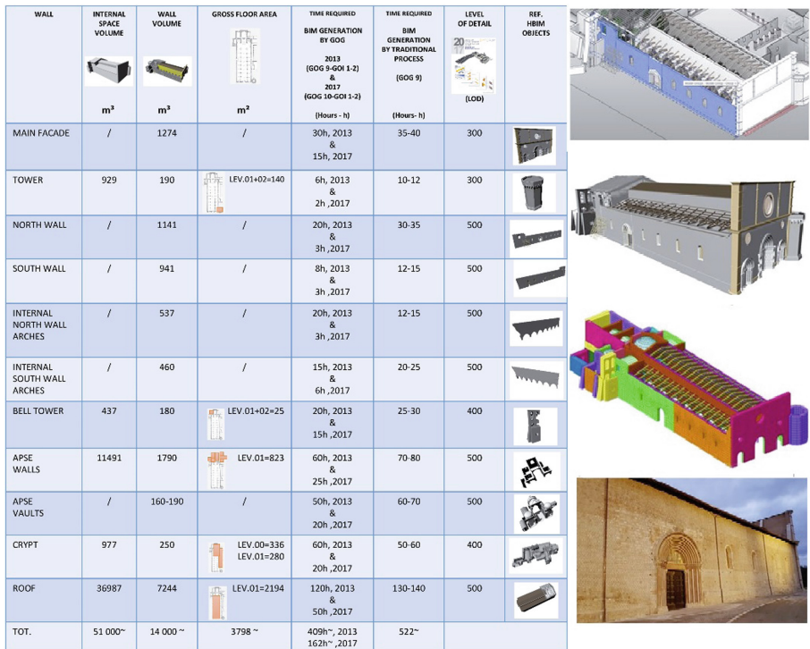
Fig. 6. The HBIM NURBS based model objects (volumes and hours effort). On the right, the case of restored north wall with the BIM to FEA (Finite Element Analysis).
